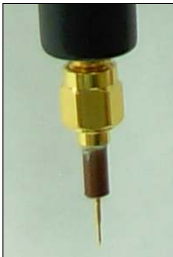
TEV NFSA Probe Antennae
