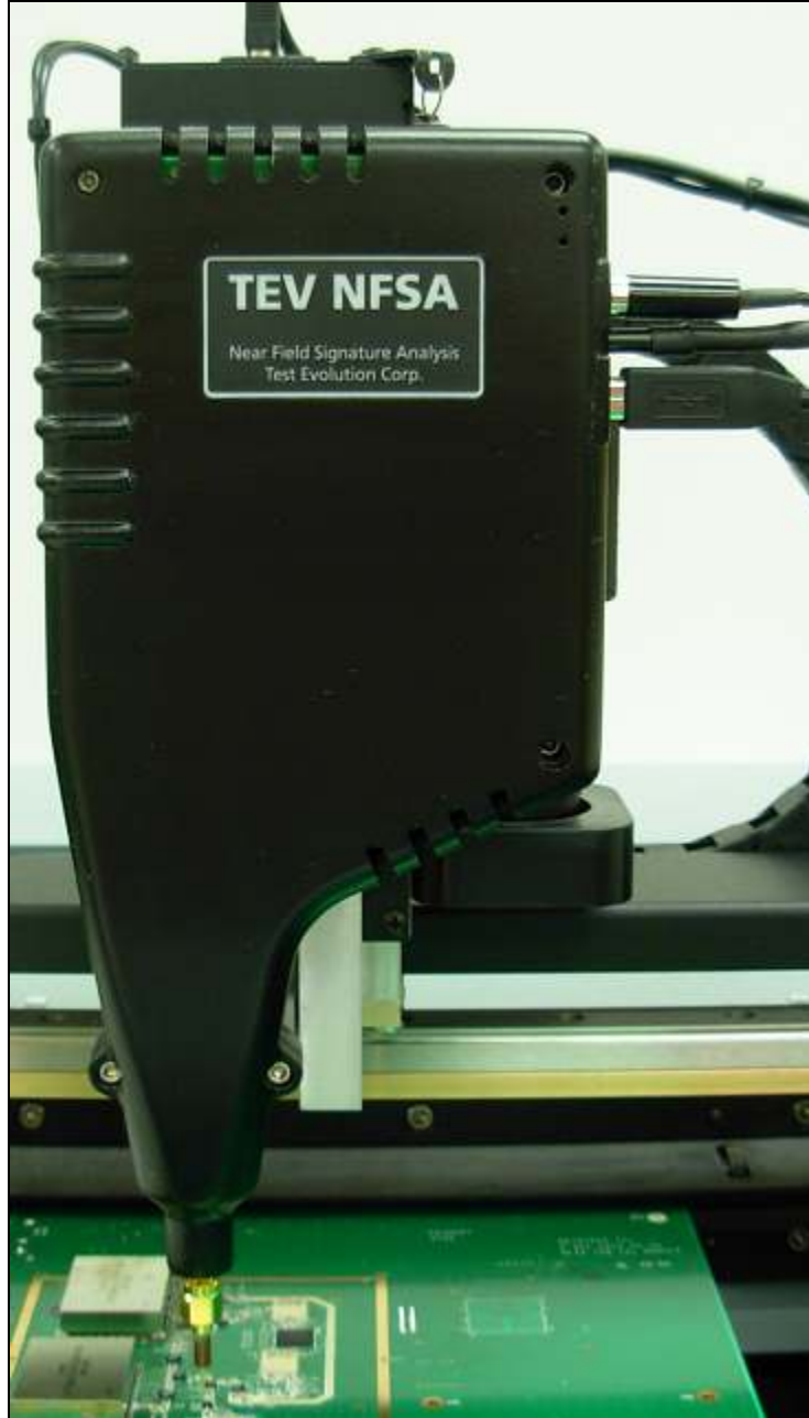
TEV NFSA Mounted on Huntron Prober
