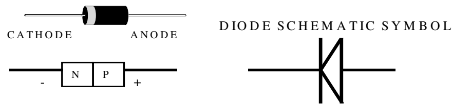
Figure 6-1. Diode and Schematic Symbol
