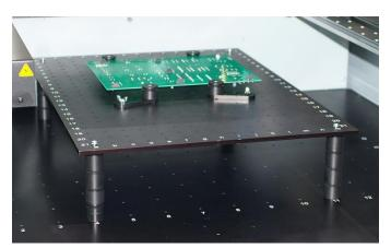
mounting of PCBs at a higher level. The plate is mounted on four Post Stacks and then additional spacers are added on top of the holding plate to secure the PCB in place. This method adds an additional degree of rigidity to the mounted board. The holding plate is 0.25" thick so the spacer sizes need to be adjusted to make up for the added height. The diagrams on the following pages showing the spacer Stack combinations include drawings using the additional holding plate
