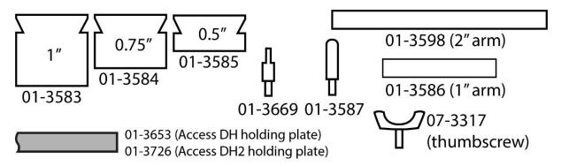
The kits pieces can be used to create a "Post Stack" which serves as an anchor support from the board edge, an adjustable "Rotating Stack" that supports the PCB from the board edge, a "Support Stack" which supports the PCB from underneath and a "Plate Stack" which uses a secondary holding plate. Use the diagrams shown on the following pages of this document to create stacks used with the Top, Middle, Bottom and Base slots of the Prober.
