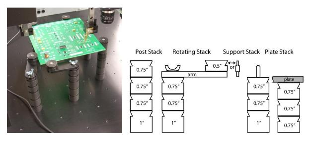
The Universal Fixture plate that makes up the support bed for the Prober has threaded mounting holes spaced at 2 inch intervals for attaching the Post, Rotating, Support and Plate stacks.
