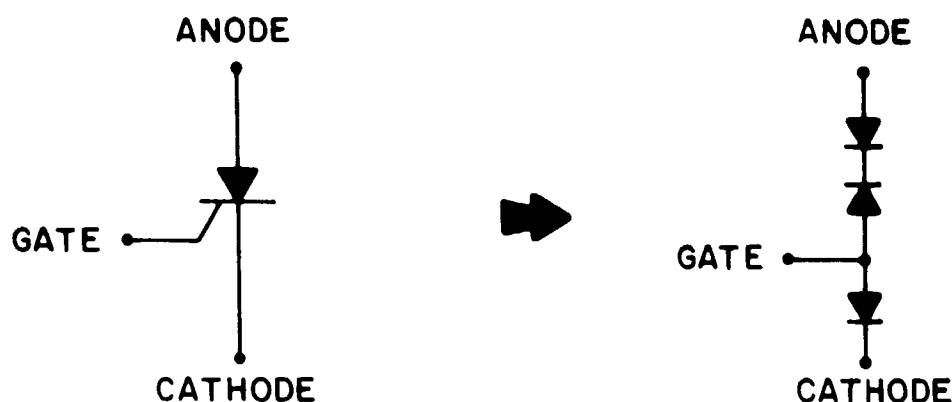
Figure 8-1. Silicon Controlled Rectifier
