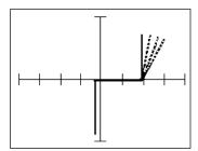
**Gap:** A missing section of a signature. Indicates a full voltage scale change during current conducting portion of the signature.
